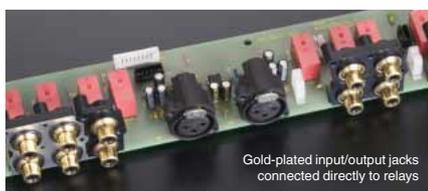
Gold-plated input/output jacks connected directly to relays
