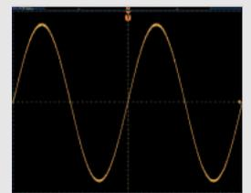
Photo (c) PS-510 output waveform (distortion approx. 0.22%)
