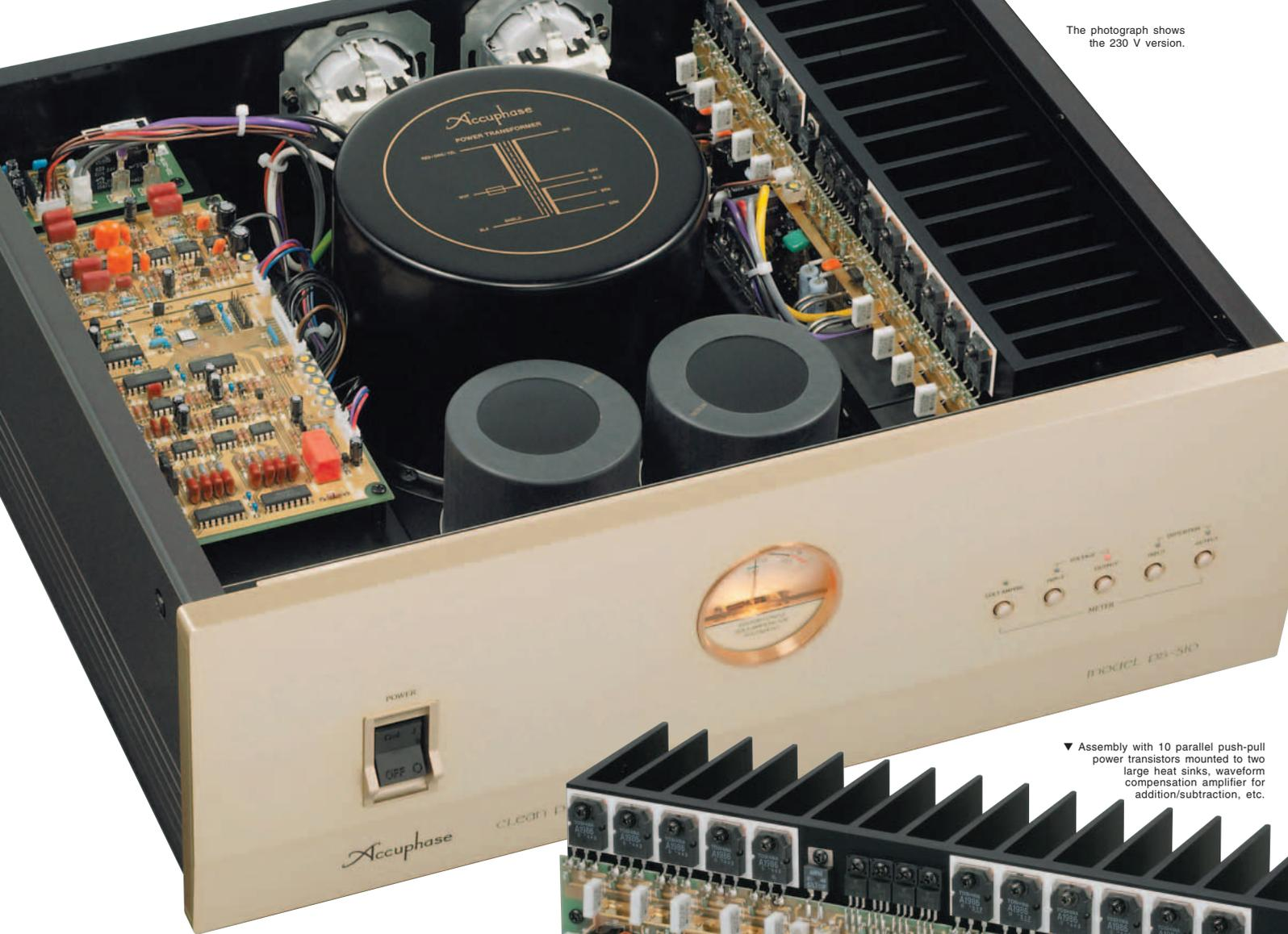
▼ Assembly with 10 parallel push-pull power transistors mounted to two large heat sinks, waveform compensation amplifier for addition/subtraction, etc.
