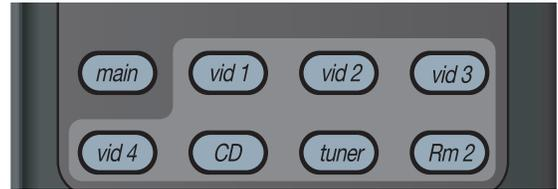
*Pressing a source button on the remote control not only selects the input associated with that source...*
