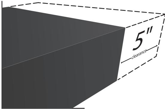
A distance of 1/2" should be maintained around the GFR-700HD for ventilation. Keep your GFR-700HD in a room where temperatures remain fairly moderate, and never cover it with table cloths, curtains, newspapers, etc., to avoid potential overheating.
