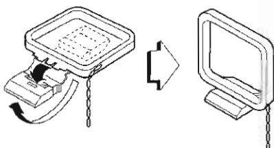
To stand the AM antenna on a surface → A
