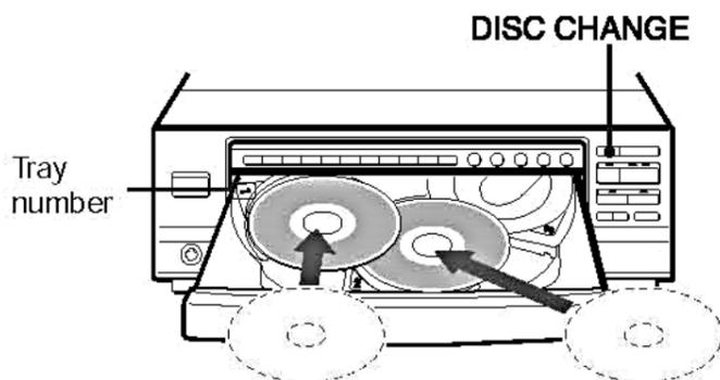
To load three to five discs, press the DISC CHANGE button to rotate the trays after placing two discs. Place the next disc on the empty tray. Each time the DISC CHANGE button is pressed, the trays rotate and one disc can be placed.
