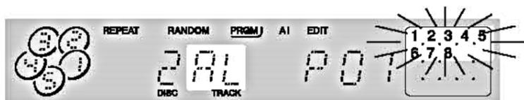
**To program a track,** press the numbered buttons and the +10 button.
