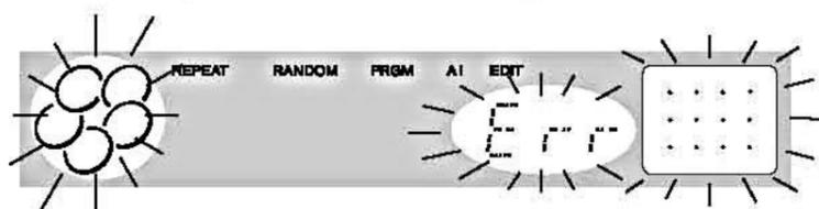
It means that an error has occurred in the movement of the disc compartment. The disc compartment may not close. A disc or something must be stuck in the disc compartment. Remove it, then press the **▲** OPEN/CLOSE button to close.
