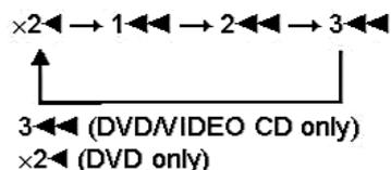
The “ $\times 2 \ggg$ ”/“ $\times 2 \lll$ ” playback speed is about twice the normal speed.
