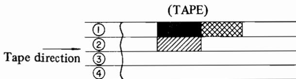
As shown in the figure, first record a 1,000 Hz sine wave on track No. 1 at +3 VU level. Next, remove the 1,000 Hz input signal and record under a non-input condition.
