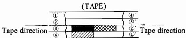
As shown in the figure, first record a 1,000 Hz sine wave on track No. 3 at +3 VU level. Next, remove the 1,000 Hz input signal and record under a non-input condition. Then, playback the tape on tracks 3 and 1 (reversed condition of tape) through the 1,000 Hz B.P.F. (Band Pass Filter, Sensitivity . . . 1 : 1) and obtain the ratio between the two by using the following formula.
