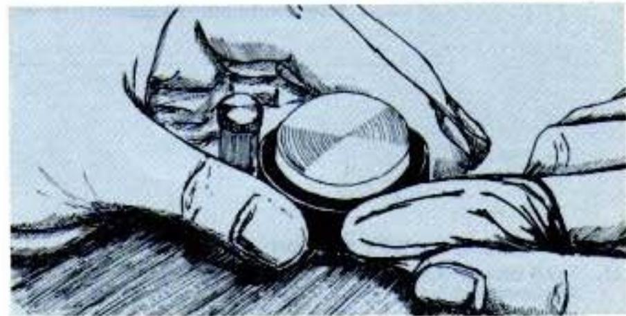
If foreign matter is allowed to accumulate on the pinch wheel and capstan, these particles will come off on the tape, causing deterioration of sound quality. Oil adhering to the capstan also causes irregularity in tape transport. It is, therefore, recommended that these parts be wiped clean periodically.
