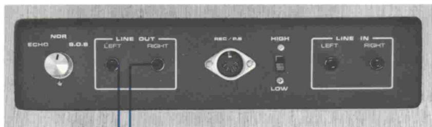
The Din Jack of the GX-400D can be used instead of the Line Output Jacks for connection with the external stereo amplifier. This enables playback or recording with a single connection cord.
