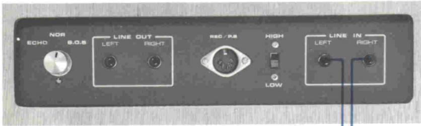
The Din Jack of the GX-400D can be used instead of the Line Input Jacks for connection with the external stereo amplifier. This enables recording or playback with a single connection cord. In this case set Din Jack Input Selector Switch to HIGH or LOW position to correspond with the output of the amplifier.
