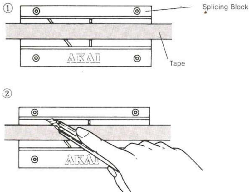
1. After marking the desired connection point, cut the tape at the mark using the standard accessory Tape Splicing Block.
