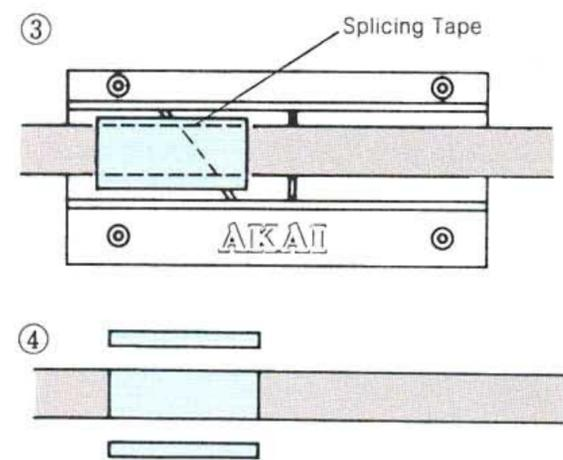
3. Tape connection is completed by cutting the excessive portion of splicing tape with a cutter.
