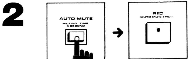
Depress the AUTO MUTE button just before the commercial starts. No recording will be made for 4 seconds. The REC ( ● ) button will flash on and off.
