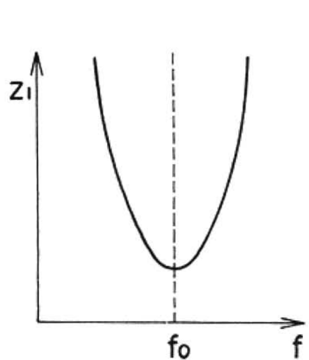
Fig. 53 B.P.F./Impedance characteristics
