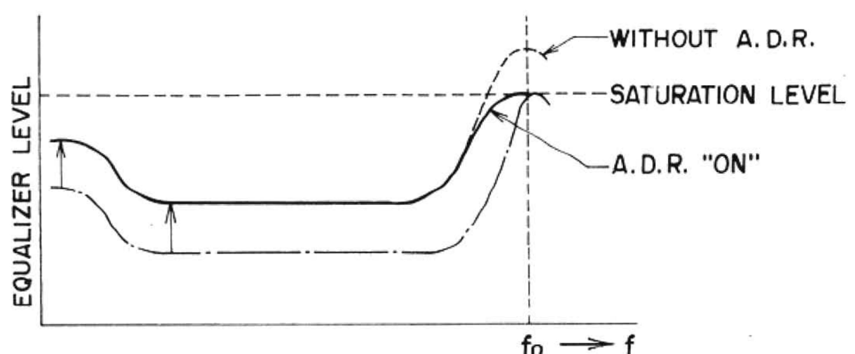
Fig. 54 Recording Equalizer characteristics
