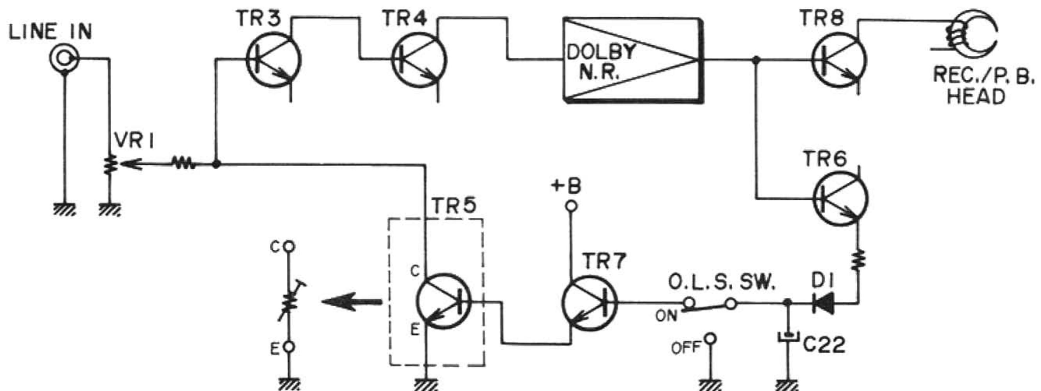
Fig. 55 O.L.S. Block Diagram
