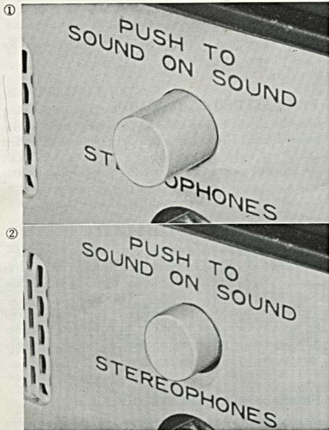
Please be sure to check and see that the push button of sound-on-sound is not remain depressed (As shown in Fig. 1) before you make a stereo recording. Should the button remains depressed recording on the right channel can not be achieved on a stereo recording. (As shown in Fig. 2)
