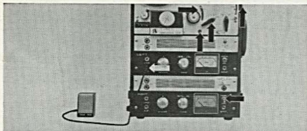
Connect a microphone to the MIC input jack of the left amplifier. To record from a radio set, record player, external amplifier, or from another tape recorder monaurally, use the LINE input jack of the left amplifier.
