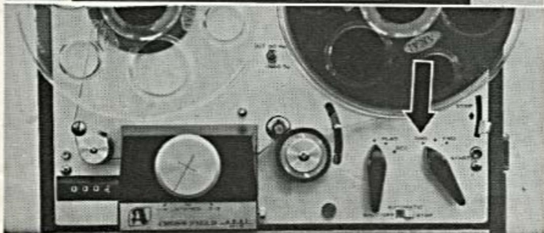
After a correct recording level is determined, push the start button to start recording on the track No. 1.
