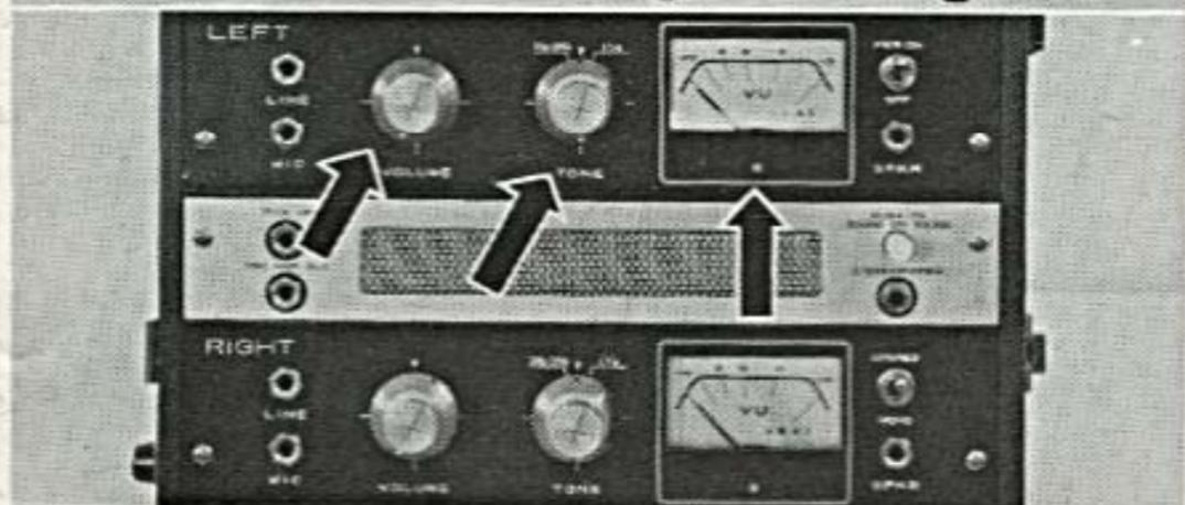
Adjust the volume control of the left amplifier to an optimum recording level while observing the VU meter. The pointer of the VU meter should not exceed the "0" level except in rare instances. The tone control has no effect when recording.
