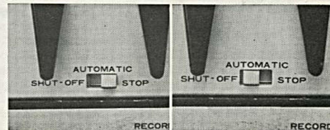
Before operating the M-8, insure that the **AUTOMATIC SHUT OFF SWITCH** is set to the position marked "STOP". The recorder will not function when the shut off switch is set to the position marked "SHUT OFF".
