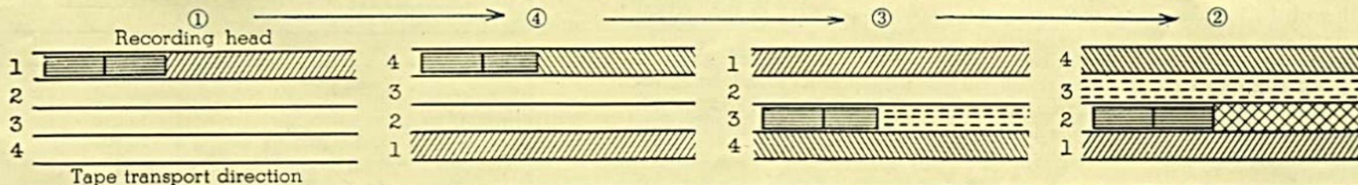
**Stereophonic recording** uses two tracks at a time, so that position reversal of both reels can be done only once, first recording on the first and the third tracks and then on the second and fourth tracks. In this case, the track selector is set to the position for stereo.
