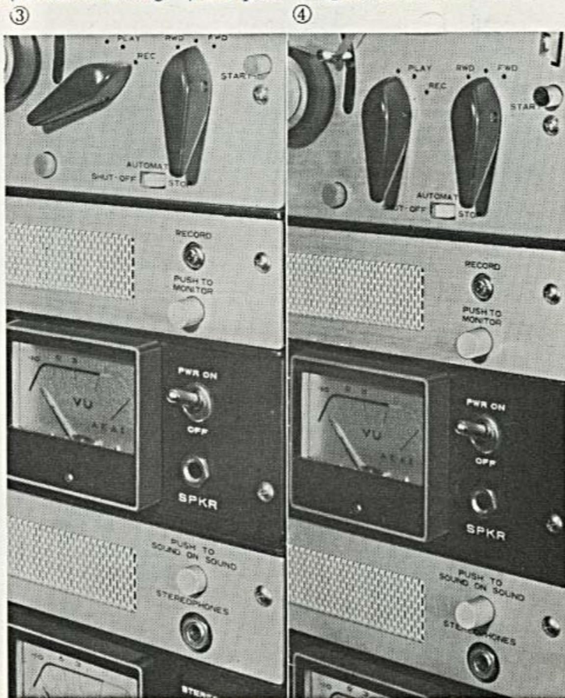
Care should be taken in order not to connect the plugs from a record player to the PICK UP JACKS. No recording can be made if plug(s) are connected to the PICK UP JACKS.
