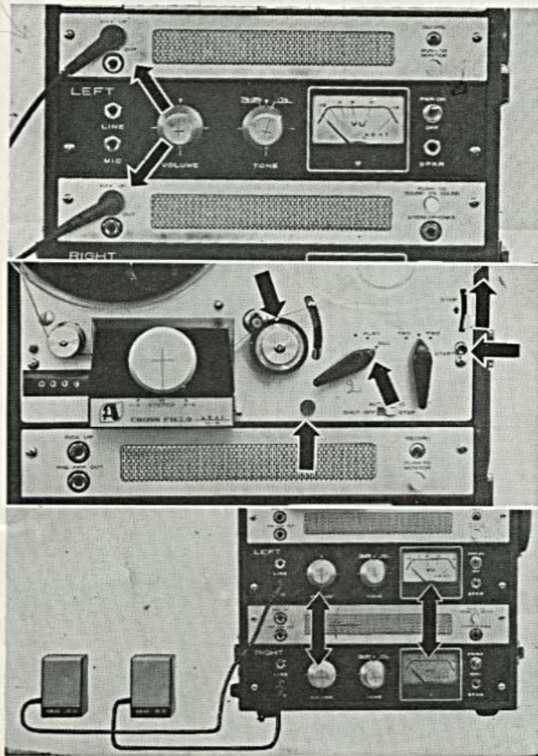
**Note:** If the microphones are used near the recorder, acoustic feedback may result. To avoid this, push the internal speaker on/off switch to disconnect the internal speakers.
