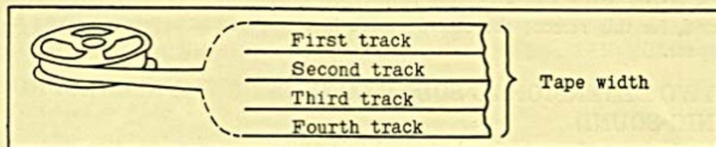
Erasing and recording/playback heads can be moved to the required track by turning the track selector knob.
