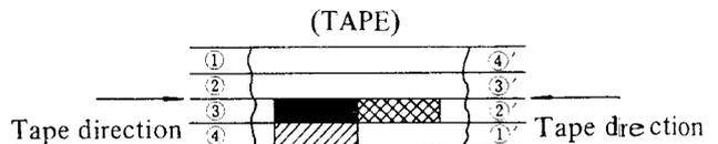
As shown in the figure, first record a 1,000 Hz sine wave on track No. 3 at +3 VU level. Next, remove the 1,000 Hz input signal and record under a no-input condition.
