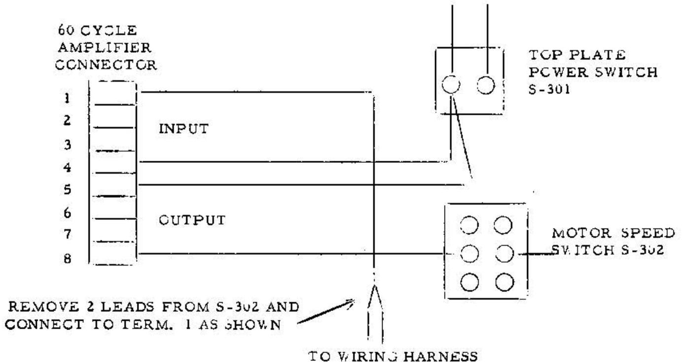
1. Disconnect the two wires from the swinger of the motor speed switch S-302. This switch has two swingers, but only one has two wires connected to it. Connect these two wires to a line leading to Pin 1 of the Model 375 input-output connector J2302P.
