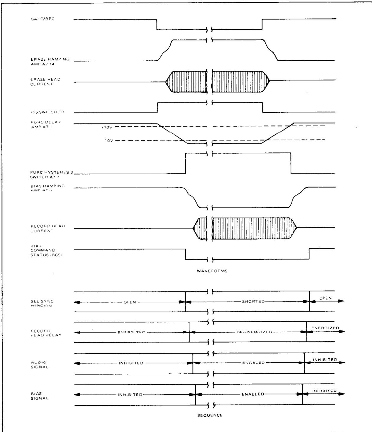
Figure 4-19. Record Ramping and PURC Delay Timing
