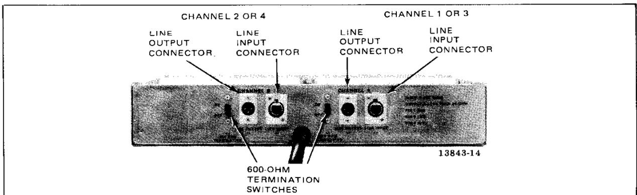
Figure 2-14. Input/Output Assembly, Rear View
