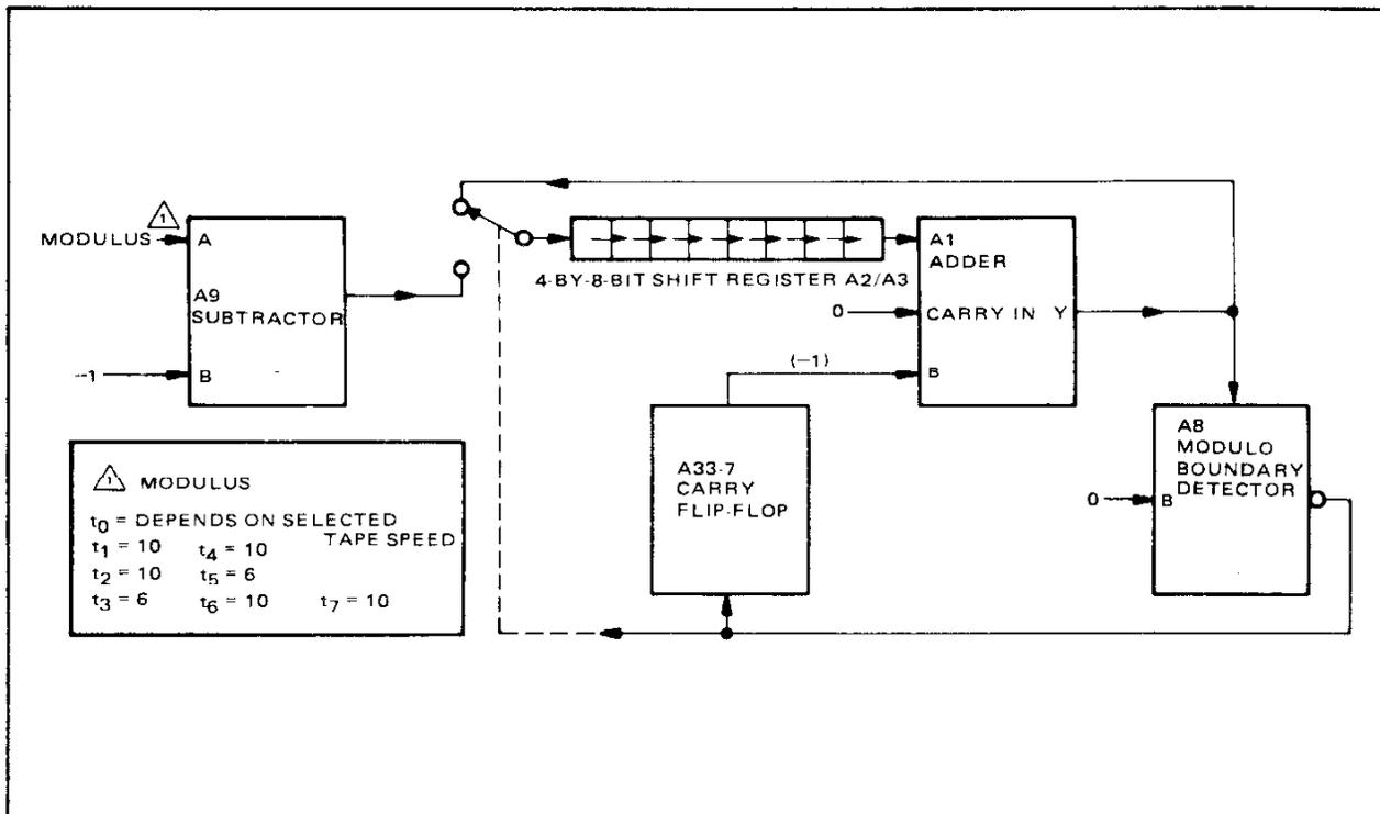
Figure 4-27. Count Down Logic, Simplified Block Diagram
