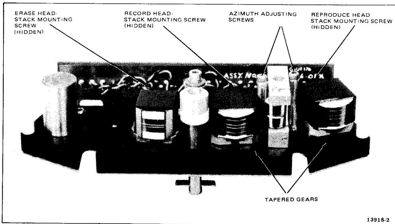
Figure 1-4. Head Assembly with Head Shield Removed
