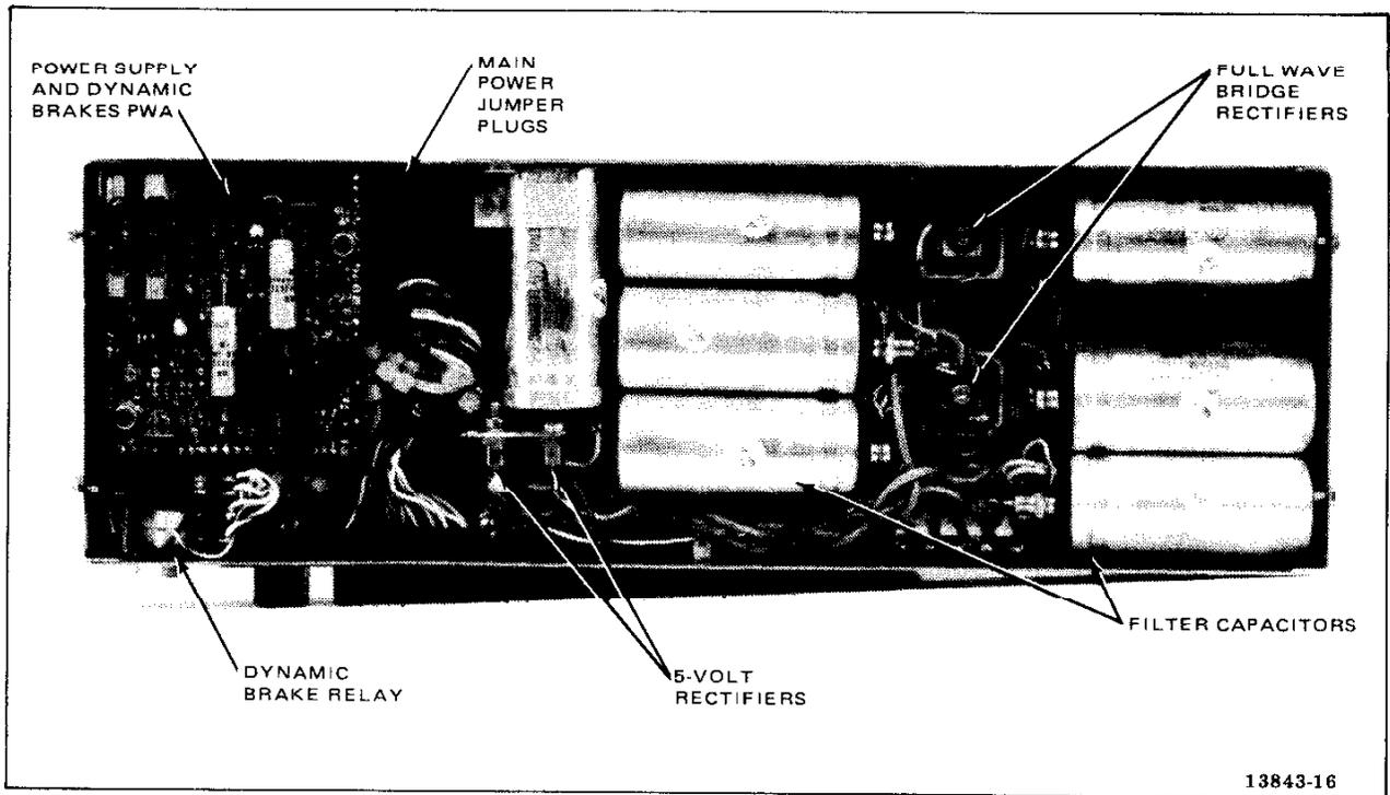
Figure 1-8. Power Supply Chassis with Cover Panel Removed
