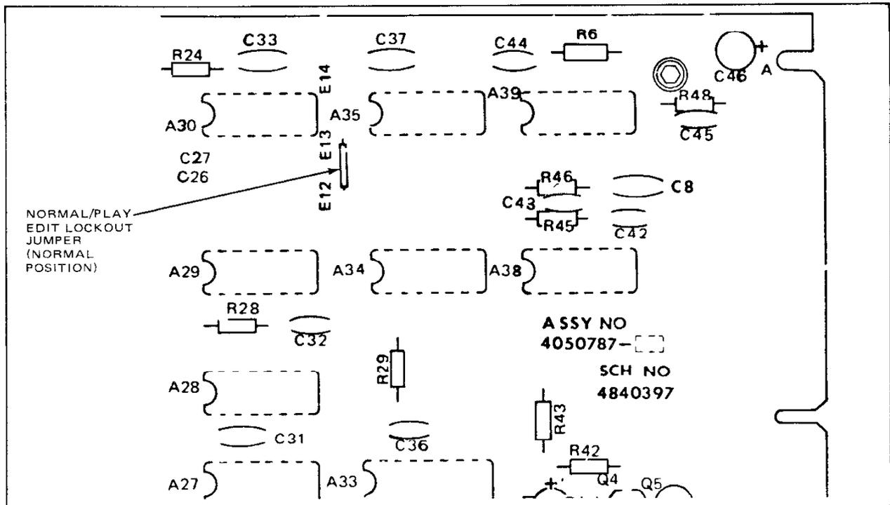
Figure 2-22. Normal/Play Edit-Lockout Jumper, Transport Control PWA No. 7
