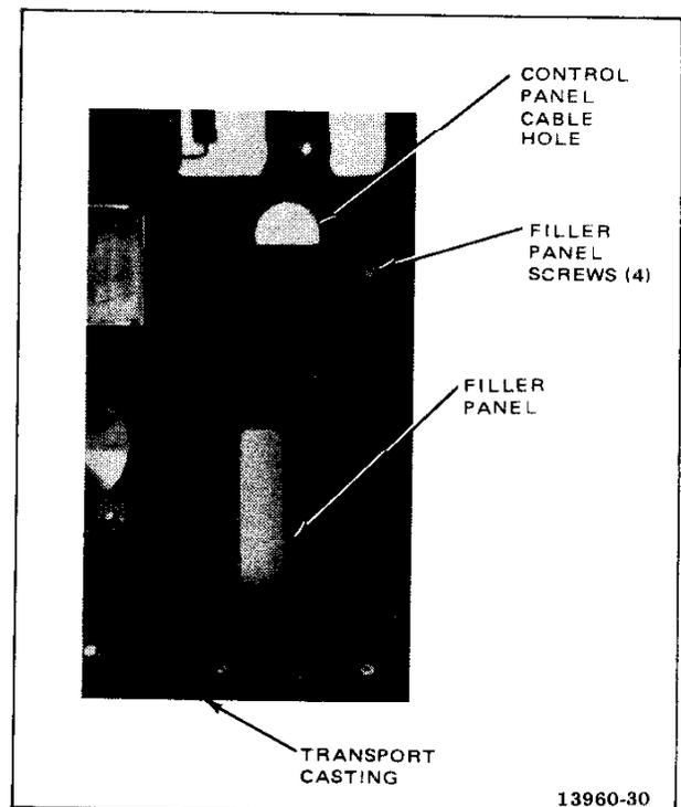
**Figure 2-20. Rear View of Filler Panel
