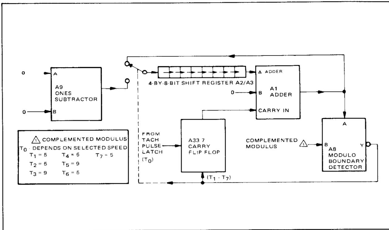
Figure 4-26. Count Up Logic, Simplified Block Diagram
