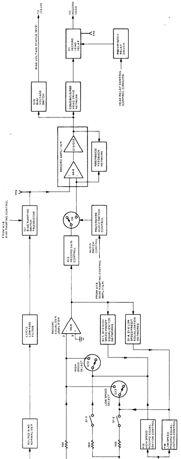
Figure 4-20. Audio Record Circuits, Simplified Block Diagram
