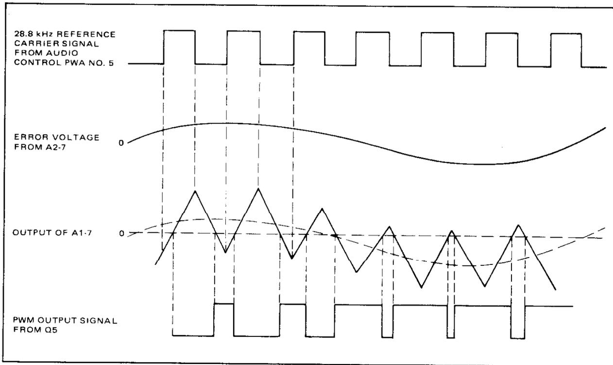
Figure 4-6. Pulse Width Modulator Waveforms, Takeup Reel Servo
