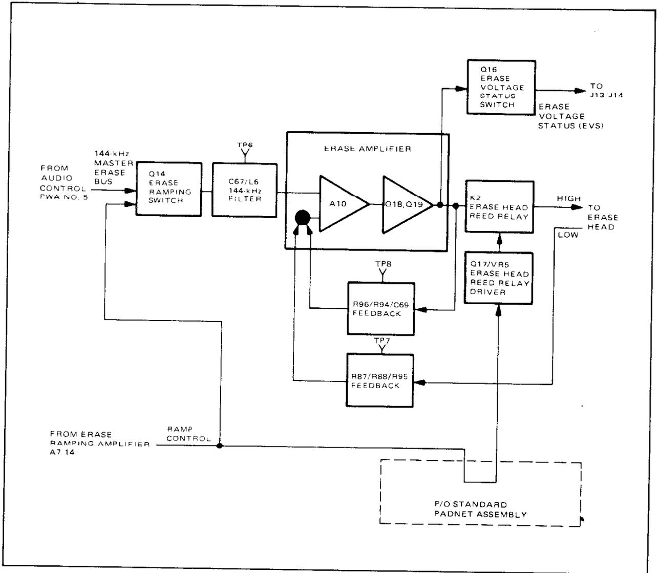
Figure 4-21. Erase Circuit, Simplified Block Diagram
