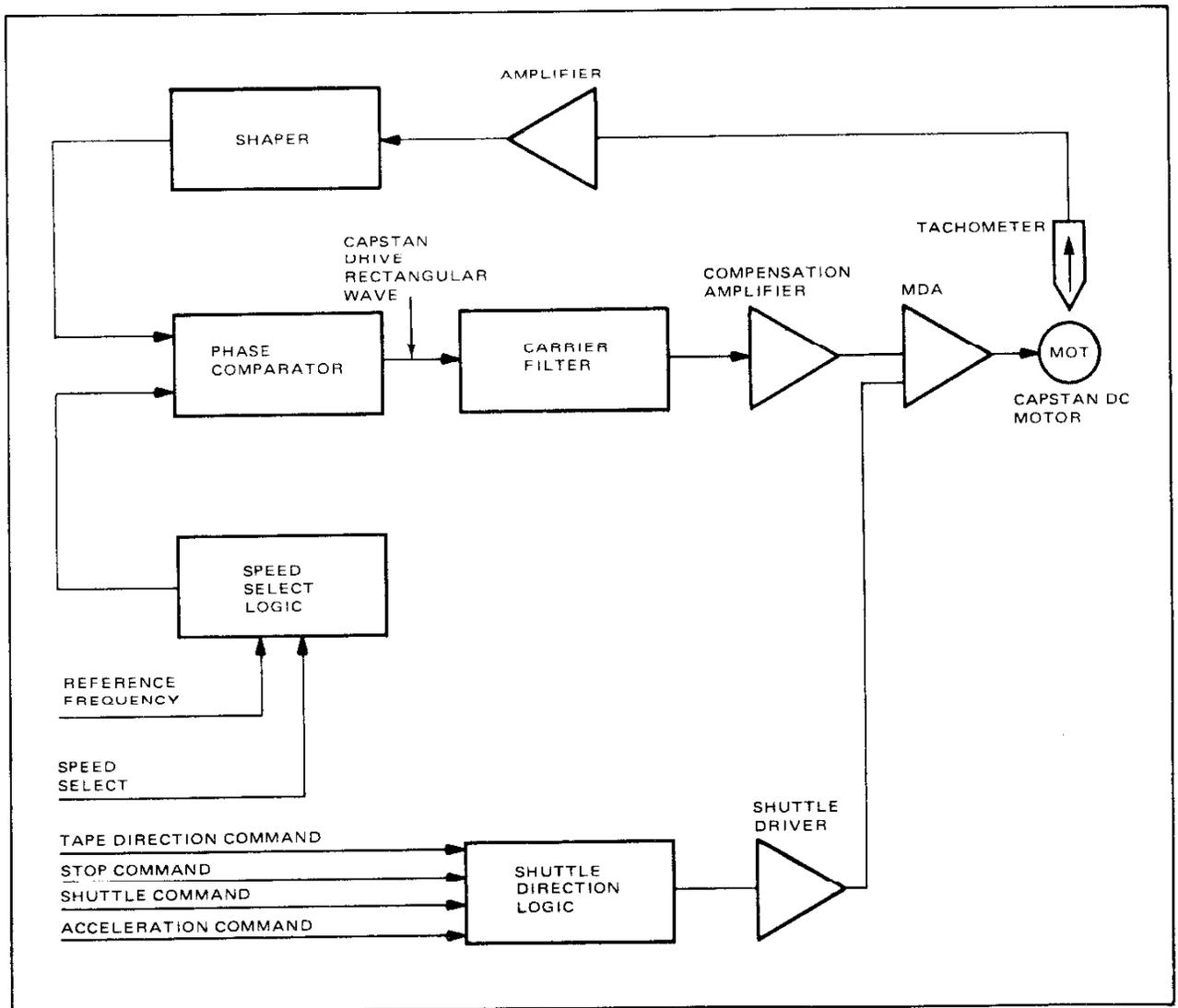
**Figure 4-2. Capstan Servo General Simplified Block Diagram**
