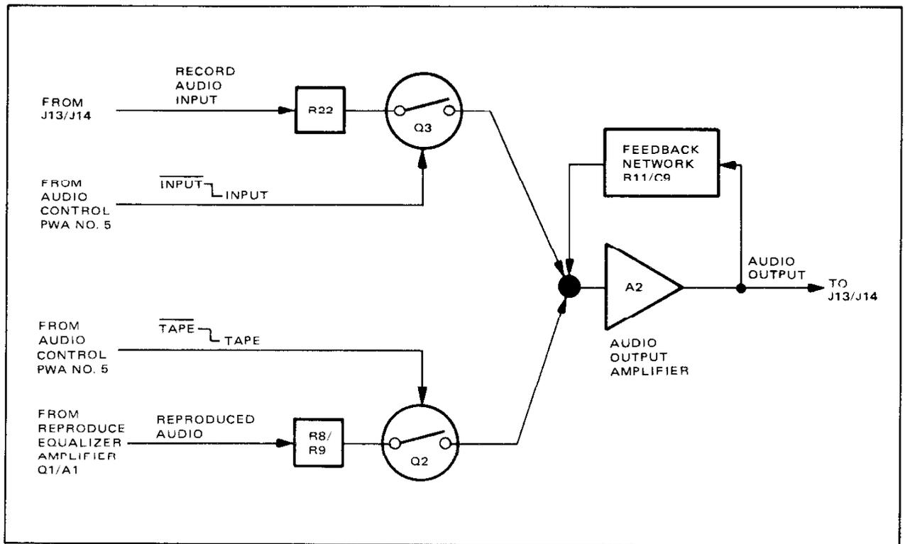
Figure 4-23. Audio Output Circuit, Simplified Block Diagram
