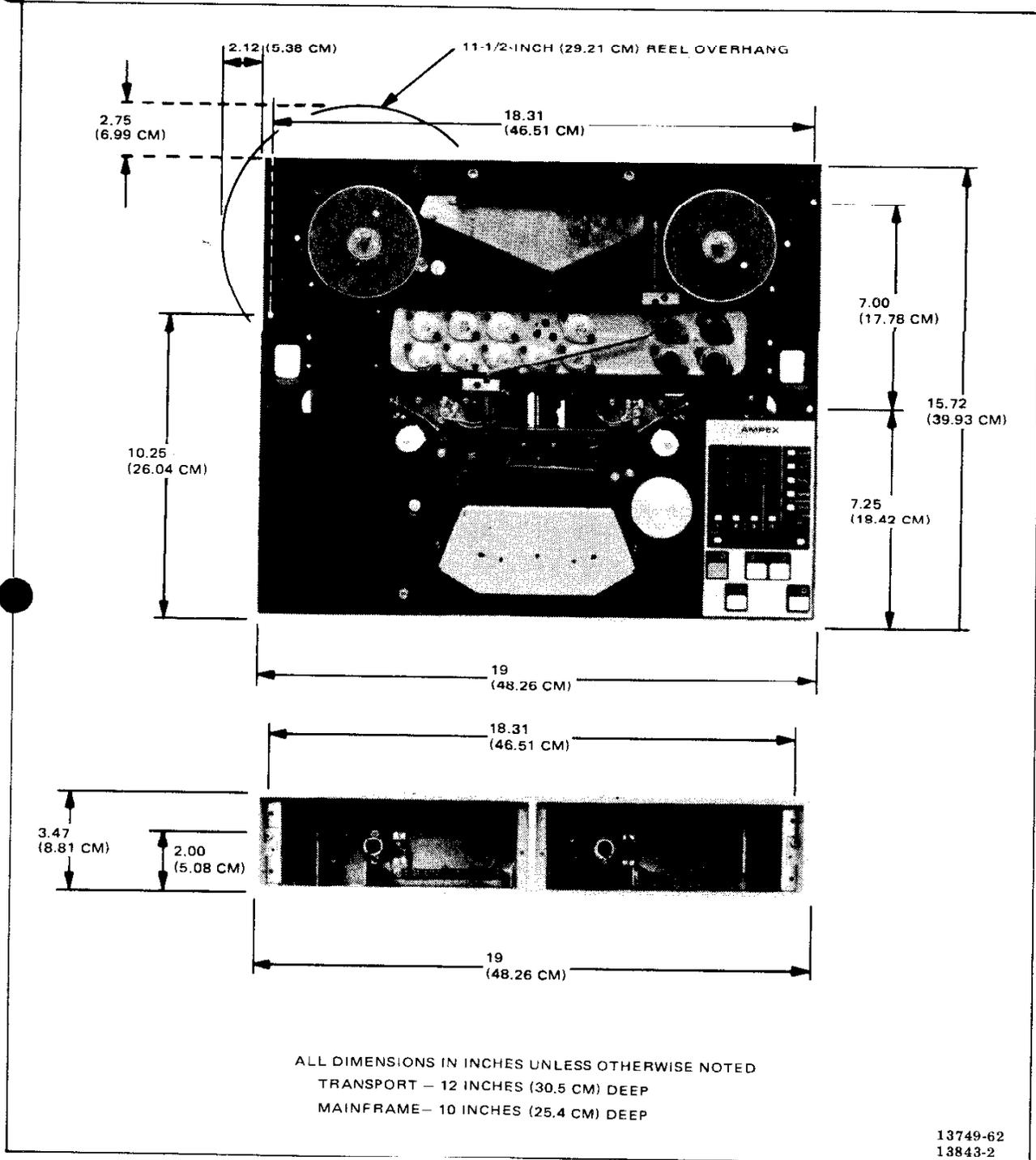
Figure 2-1. Mounting Dimensions
