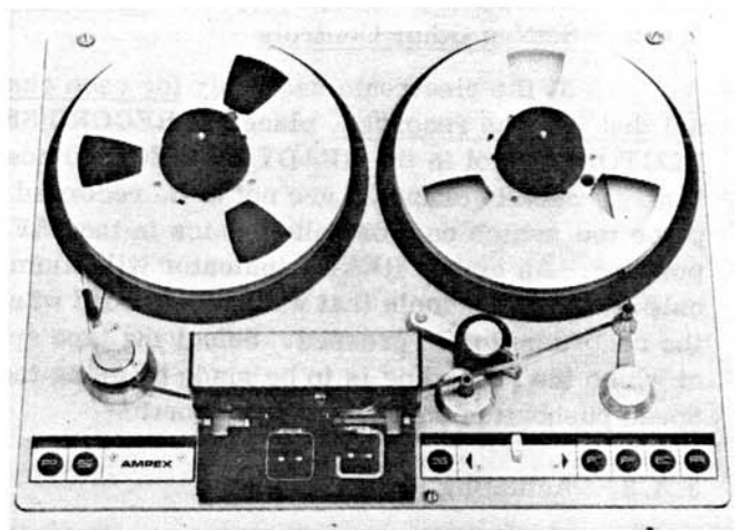
Fig. 3-3. Tape Threading Path
