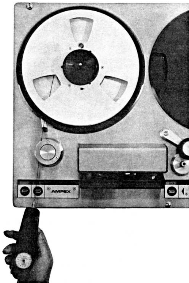
Fig. 4-2. Checking Holdback Tension
