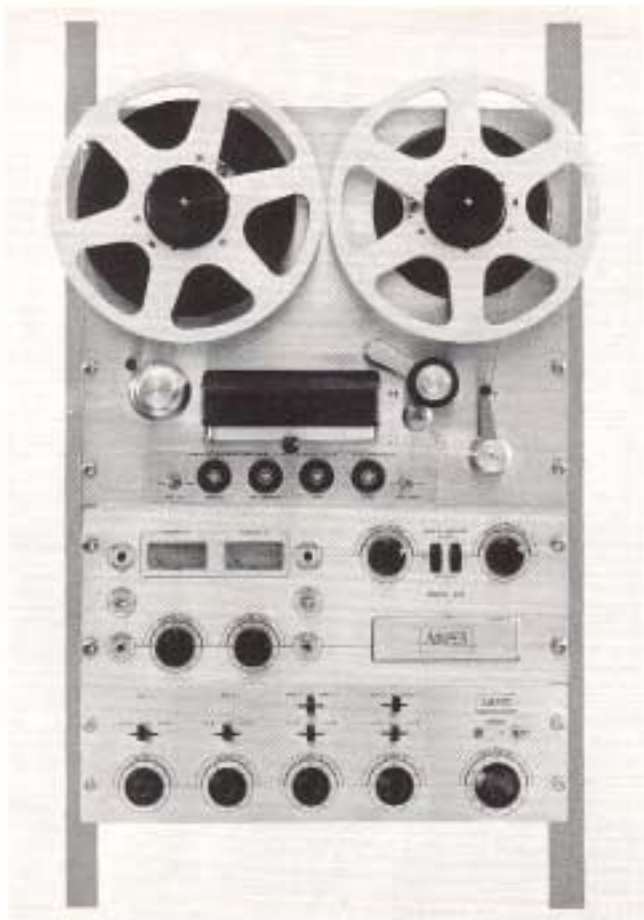
Rack layout (shown with Ampex 354 tape recorder)
