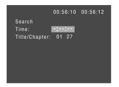
If the disc is playing, then the elapsed and total times on the disc are shown in the top right of the page.
