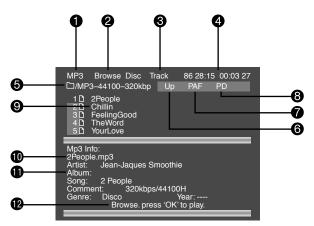
The screen shown above is the disc navigator screen, in this example showing a CD-R containing MP3 files. The following items can be identified:
