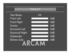
The relative sensitivity (volume) of different speakers can lead to some speakers sounding disproportionately loud or quiet, relative to others in the system. The trims setting of your DV89 can help to address this inbalance.
