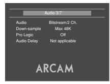
This section allows you to configure the type of analogue and digital audio outputs. In particular, the digital output type needs to be set correctly if you are using an external audio decoder, receiver or D-A converter.
