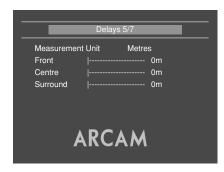
The relative positioning of speakers within a room (particularly a large room) may mean that sound from some speakers arrives at the listener later than sound from others. By altering the delay settings for the different speakers, this difference in arrival time can be reduced or eliminated.
