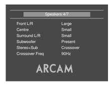
This menu screen allows you to specify the speaker configuration that is connected to the analogue ouputs of your DVD player. (Note that these settings do not affect the digital output in any way.) It is important that this configuration accurately reflects the actual situation, otherwise audio quality may be severely compromised.
