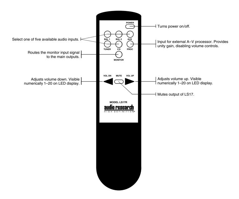
**NOTE:** All LS17 functions are available on the LS17R hand held remote controller. All functions are indicated on the front panel as they are selected. See "Description of Controls" in this manual for more information.
