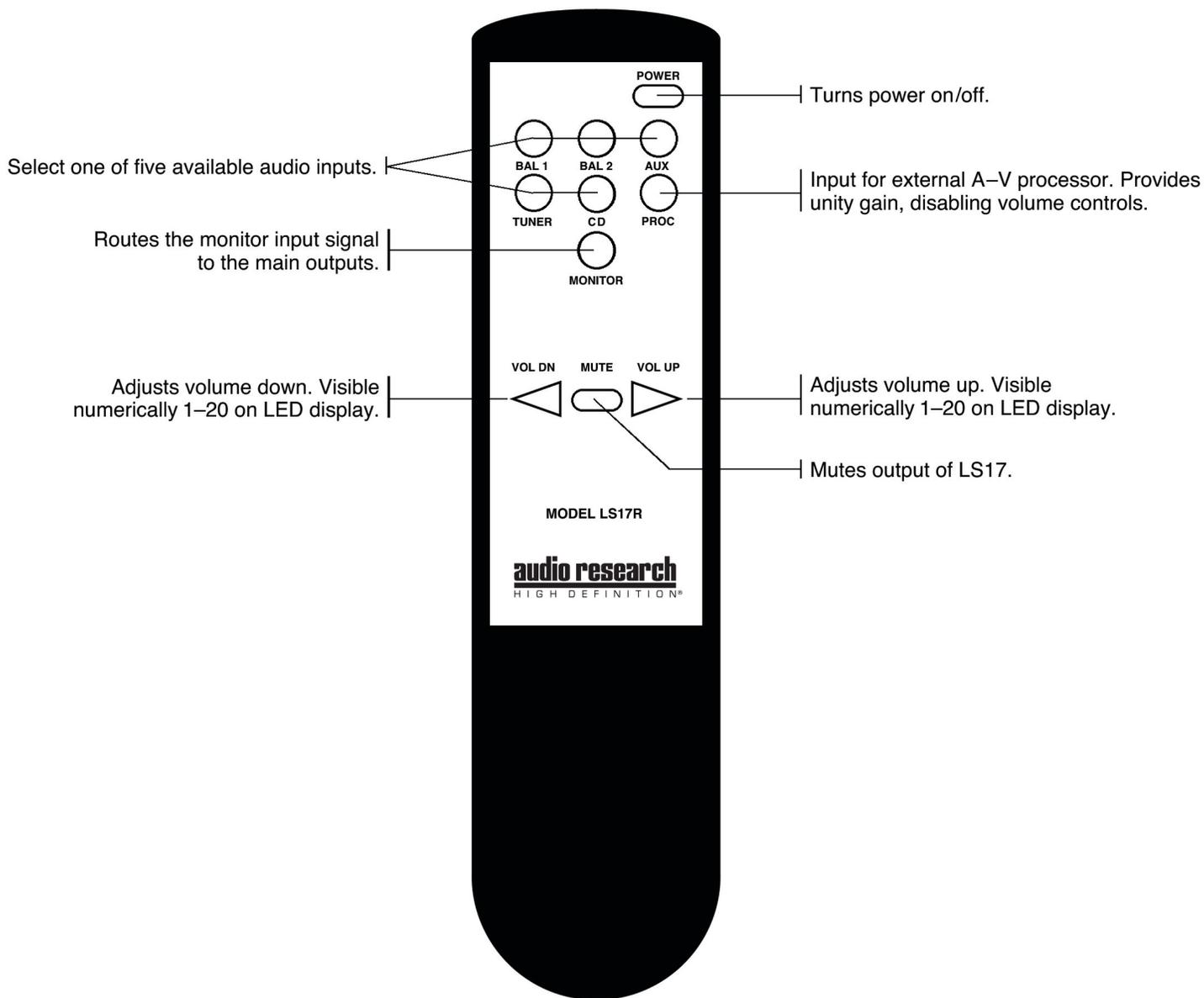
NOTE: All LS17 SE functions are available on the LS17R hand held remote controller. All functions are indicated on the front panel as they are selected. See 'Description of Controls' in this manual for more information.
