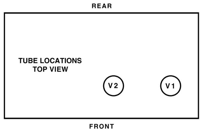
Diagram indicates relative positions of two 6H30 tubes located on circuit board as viewed from the front and looking down from above the preamplifier.
