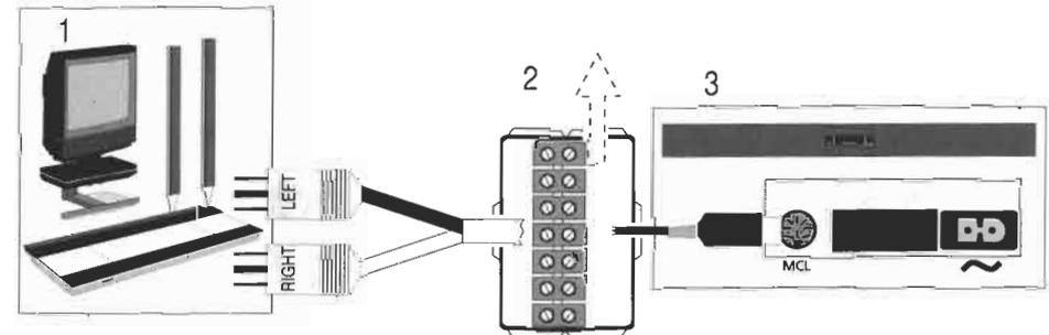
*Connecting and installation of the the LCS 9000 for a Local room is very easy as shown in the illustration*
