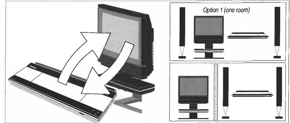
*In stand-by, press SOUND, then 2, STORE, and the Beocenter 9300 is programmed to Option 2, in stand-by, press PICTURE, then 2, STORE, and the Beovision is programmed to Option 2. If the system is to be reprogrammed to AV integration in one room, the procedure is the same, just select 1 for both masters. Note: The above is Beolink 1000 operation only.*
