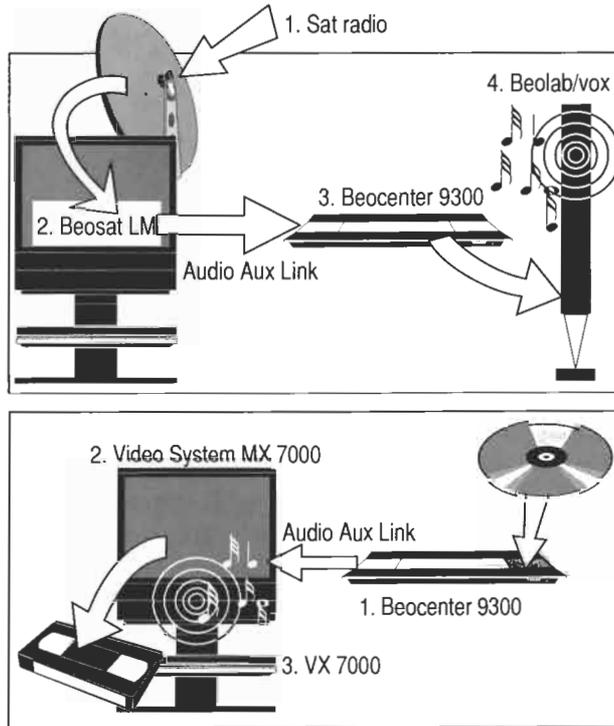
impressive sound image) either as an accompaniment to the video on the screen, or with inactive screen, if you only want the music. Reception of satellite radio with reproduction via the speakers of the audio system and inactive screen is another logical option in a Beolink AV system.
