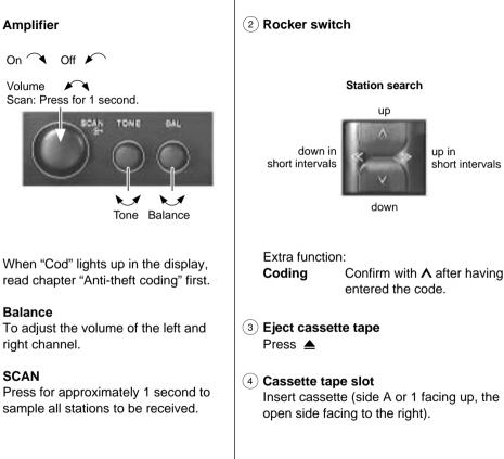
Rapid tape run/Autoreverse (5) Switch-over to the other track Press simultaneously Fast Fast rewind: forward: To stop: press FF To stop: press FR Side A or 1 Side B or 2 Track indication 6 Display Wave band Frequency Memory bank Preset button - ARI priority - ARI 6.5 SK station code Stereo Sensitivity (station search)
