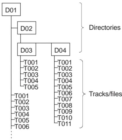
Each directory can be named using a PC. The directory name can be displayed in the device's display. Name the directories and files using your CD burner software. The software's operating instructions will provide details on how to do this.
