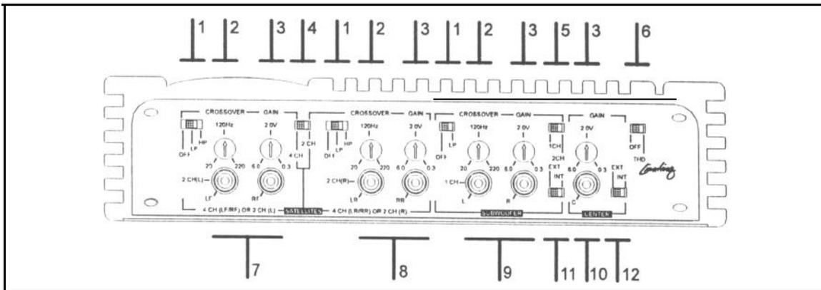
1. CROSSOVER FREQUENCY CONFIGURATIONS - In the full-range mode (5-50,000 Hz) the amp reproduces all frequencies heard by humans. In the LP (low-pass) position, only low frequency (bass) comes out of the speakers. In the HP (high-pass) position, only information above the crossover frequency setting is sent to the speakers.
