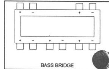
3. **EC-1, END CAP:** If only one amplifier is installed in a car, these end caps can be placed at either end of this amp to protect the control settings and wires. If two or more amps are used, an EC-1 can be mounted between two amps to "bridge" the gap between the two amps thus trimming out the appearance nicely.
