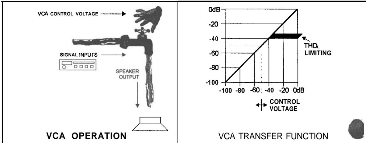
Many people want to have a remote control for a high power amplifier in order to control the loudness of a subwoofer amplifier independently of the radio. Remote mounting of an input gain control would be a major problem with most car audio amplifiers because of the likely noise intrusion into the signal path.
