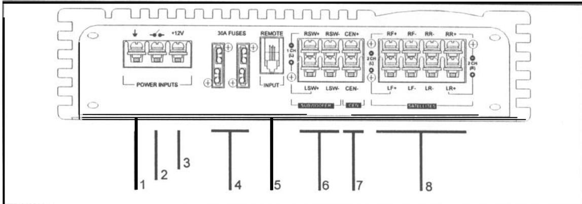
1. **GROUND LINE** - This is the high current ground connection to the chassis of the car. It should be fastened to a clean ground connection in the car, capable of handling high current loads. Do not run a wire up to the car battery ground for this line. It should remain less than 3 feet in length (1meter).
