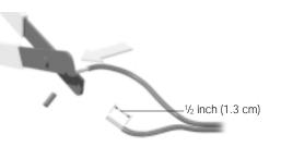
At the ends of each cord, strip approximately  $\frac{1}{2}$  inch (1.3 cm) of insulation from both wires (Figure 14). Next, twist the ends of each wire so there are no loose strands.
