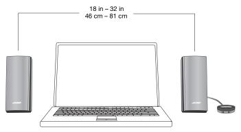
The size and shape of these speakers make it easy to position them directly next to your computer. To provide an accurate sound stage, you should observe the following guidelines:
