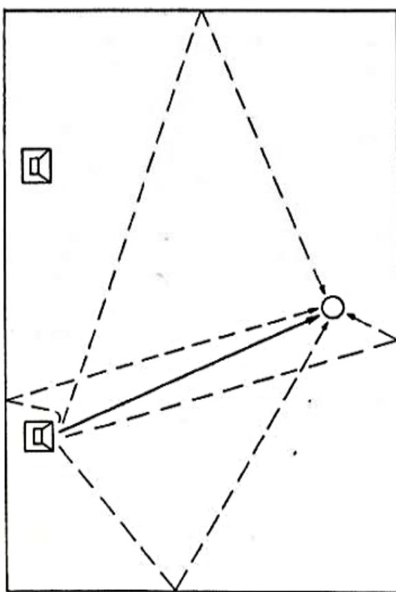
This sketch shows a better arrangement of the speaker in the same 12 x 18 foot room; the speakers are now five feet away from the side walls, substantially weakening the mirror-image wall reflection and moving it six milliseconds later in time where it becomes innocuous. The speaker has also been pulled forward from the wall a few
