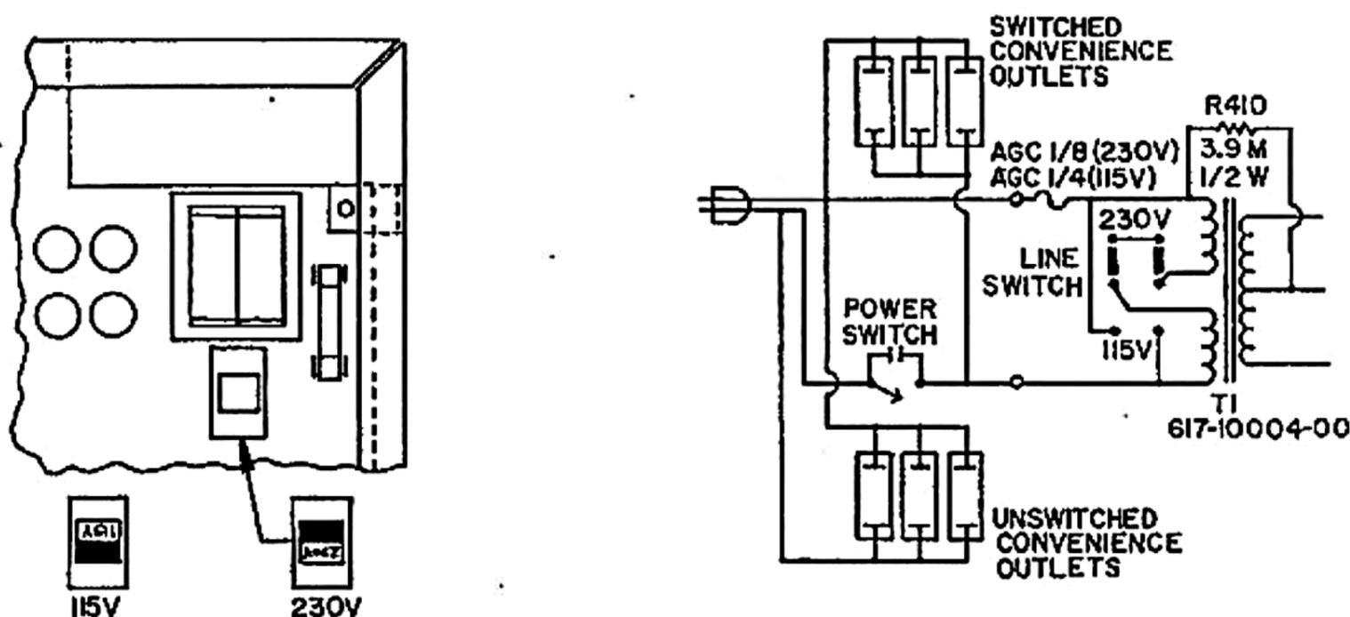
Figure 8-1. 115/230 Line Voltage Conversion Switch & Fuse
