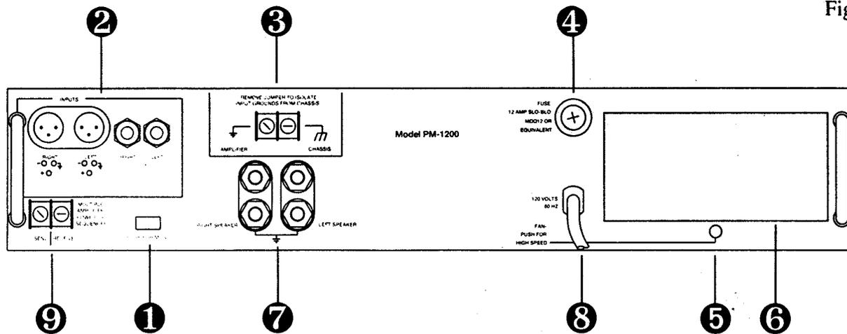
4. FUSE. AC power line fuse for the PM-1200. Use only one of the following fuses for 120-volt models of the PM-1200:
