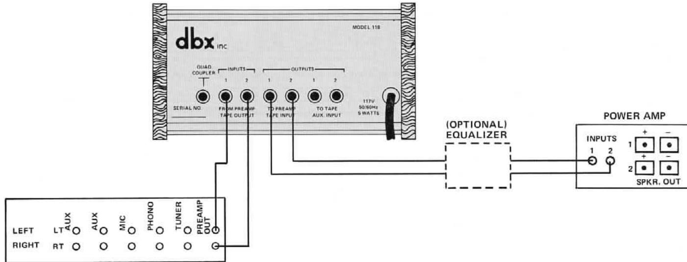
Fig. 6 — Installation of a dbx 118 in a Sound System where the Preamp has no Tape Monitor Loop, and a separate Power Amplifier and Preamp/Receiver are utilized. This same setup applies where an Integrated Amp/Preamp or Receiver has Preamp Out/Main Amp in Jacks.
