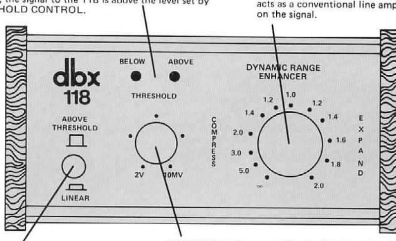
**ABOVE THRESHOLD/LINEAR (Switch)** When in the LINEAR position (switch "in"), the 118 functions over the entire range of input signal levels. When in the ABOVE THRESHOLD position (switch "out"), the 118 acts only on signals above the level set by the THRESHOLD control. (Refer to Figure 3, B & D.)
