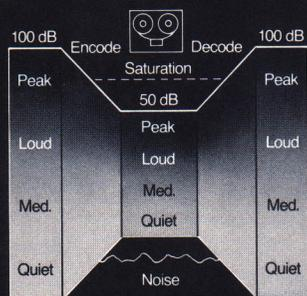
dbx II tape noise reduction uses 1:2 compression to enable you to fit your music onto tape above the noise level, and below saturation; it then uses 2:1 expansion to restore dynamic range, with no audible tape noise added by the recording process.
