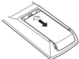
② Load the two batteries properly as indicated by the marks in the battery compartment.
