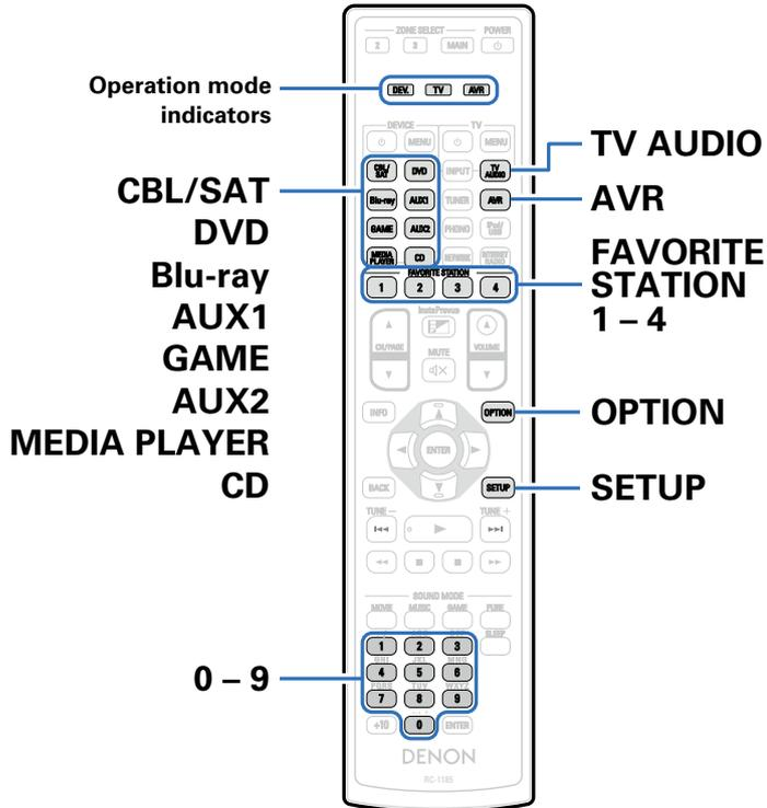
When preset codes are registered in the included remote control unit, it can then be used to operate any devices you have, such as DVD players or TVs made by different manufacturers.
