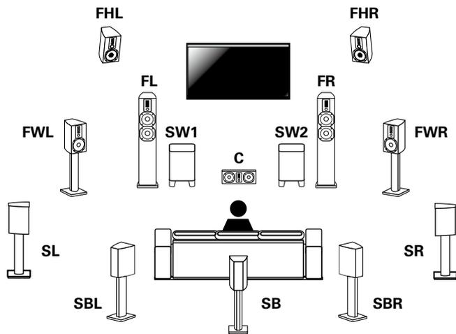
**FL/FR** : Place the FRONT left and right speakers an equal distance from the main listening position. The distance between each speaker and your TV should also be the same.
