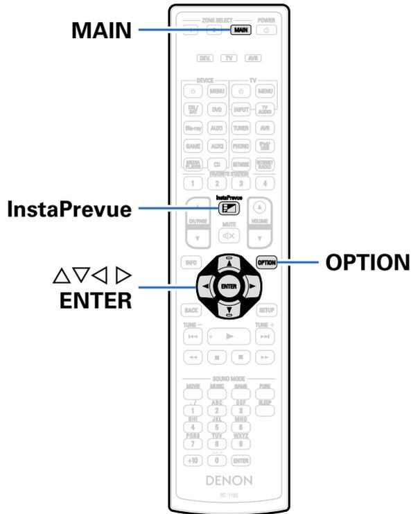
You can display sub screens on the main screen to preview playback video of the HDMI input connected to this unit. You can also display various video inputs in a single screen to switch input sources such as Blu-ray, DVD, and GAME while viewing them on sub screens.
