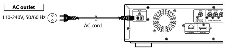
**Supplied cables used in this connection are as follows:**
