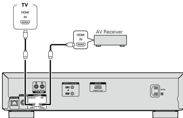
The MONITOR(VIDEO) connector outputs video signals.
