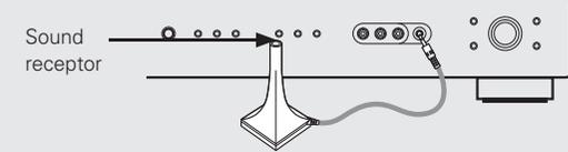
**3** Place the microphone at ear height on a tripod or stand with the microphone pointing directly up towards the ceiling.
