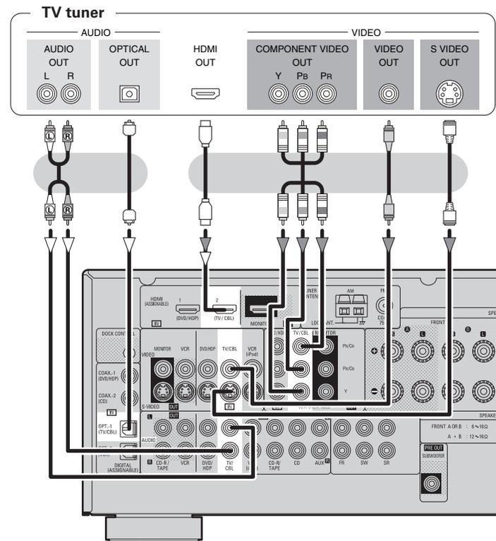
When using a coaxial cable for the digital audio connection, make the settings at "System Setup" – "Input Setup" – "Digital In Assign" (page 21).
