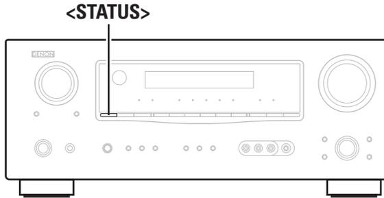
Information on the main unit’s various settings (Status) and on input signals (Audio Input Signal) is shown on the display. The information displayed changes each time you press **<STATUS>**. The information is displayed for several seconds before the display returns to its original condition.
