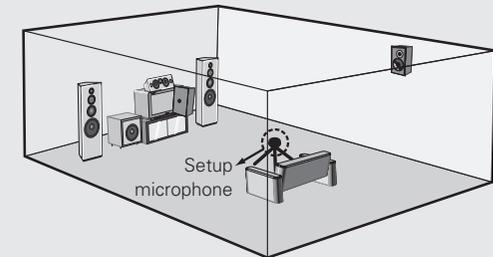
※ Do not hold the microphone in your hand during measurements. Be sure that the path from microphone to the speakers is not blocked by objects. Avoid placing the microphone close to a seat back or wall as sound reflections may give inaccurate results.
