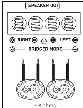
Typical Stereo Wiring
