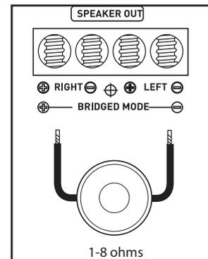
Typical Bridged Wiring
