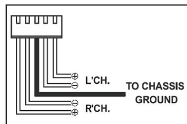
**Note:** Do not use both low and high level inputs at the same time - connect only one or the other. High level inputs not available on AX3000M, AX4000M and AX5000M..
