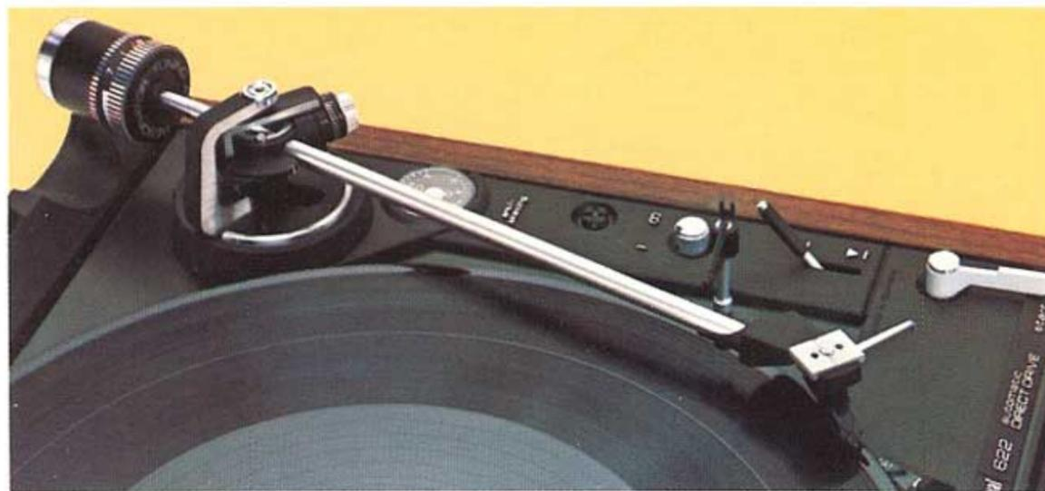
The potential for an Ultra-Low-Mass system has long existed in Dual's straight-line tubular tonearm with its four-point gyrosopic gimbal suspension. The tonearm mass is centered at the pivot point. The vernier-adjustable counterbalance establishes zero balance with micrometer-like precision. A tempered flat-wound spring applies tracking force directly at the pivot—without increasing effective mass.
