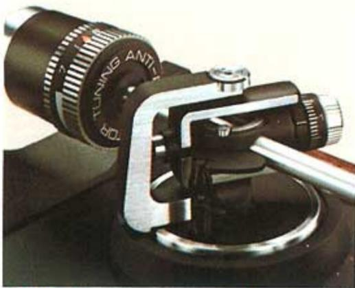
All Dual tonearms are mounted in this four-point gyrosopic gimbal. Tonearm mass is centered and pivots precisely where the vertical and horizontal axes intersect.
