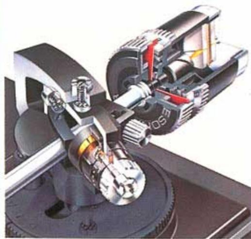
All Dual tonearms are mounted in this four-point gyroscopic gimbal. Tonearm mass is centered and pivots precisely where the vertical and horizontal axes intersect.
