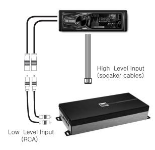
**Note:** Do not use both low and high level inputs at the same time - connect only one or the other.
