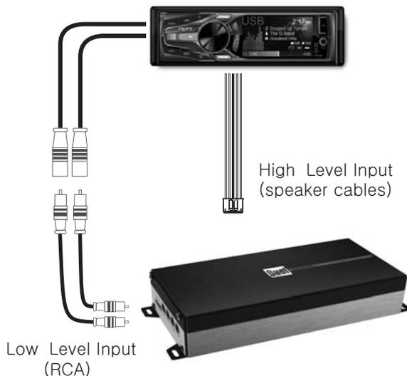
**Note:** Do not use both low and high level inputs at the same time - connect only one or the other.
