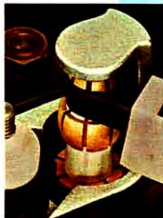
Gimbal-mounted Dual tonearms pivot horizontally and vertically on identical sets of pivot points and high-precision low-friction bearings. The metal of the pivot point is first hardened and then honed, a process which produces microscopically smooth surfaces. The ball-bearing races are only 0.157 inch in diameter. Note position of stylus-pressure spring around vertical pivot.
