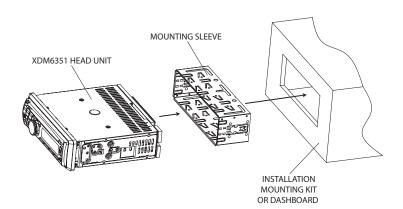
TYPICAL FRONT-LOAD DIN MOUNTING METHOD
