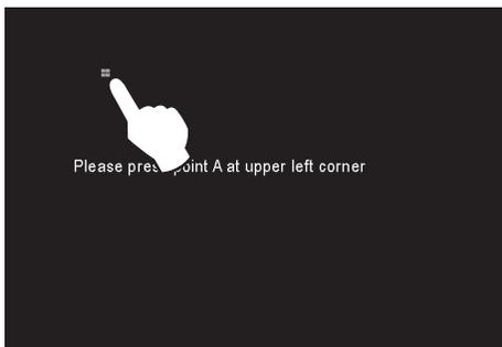
5) Touch and hold the pointers as indicated on the screen for 2 seconds each
