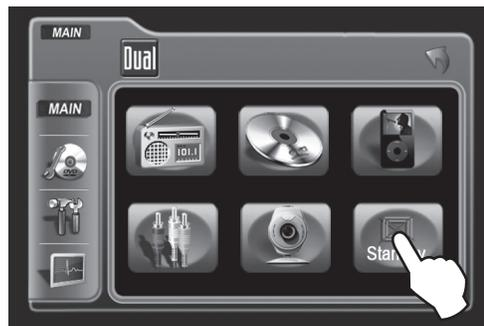
To conserve the LCD backlight lifespan or to eliminate glare while night driving, press STANDBY. The TFT screen will black out, however all other operations continue to operate. Press any button except **VOLUME** or touch the screen again to return to normal viewing.
