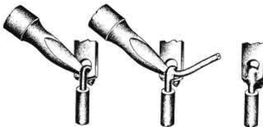
One of the best ways to make a good mechanical connection is to bend a small hook in the end of the wire, and then to crimp the hook onto the terminal lug. The amount of bare wire exposed need not be exactly  $\frac{1}{4}$ -inch, but if it is too long, the excess might touch another terminal lug or the chassis. Do not wrap the wire around the lug more than one time, as this makes the connection difficult to remove if an error is made.
