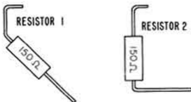
15( ) Select the remaining 150 ohm resistor; bend and cut its leads as shown for Resistor #2. Connect the lead with the bend at the end to lug #12 (S-2). Orient the resistor correctly for connection to HJ lug #1.
