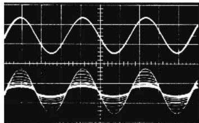
Onset of Dynaguard-20 on 200 watt signal 150 Hz
