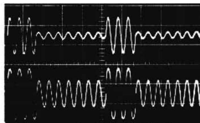
With Dynaguard-20 locked in, a 200 watt signal is limited, while an alternate 7 watt signal is totally unaffected. This preserves the essential signal characteristics, and does not reduce the dynamic range as a compressor does. Input signal above. In this example, the (upper) input signal would normally drive to an average rms output of 68.5 watts. Dynaguard limits it to an average rms output of 13.8 watts. An equivalent input for 200 watts average would yield a 20 watt Dynaguard average level.
