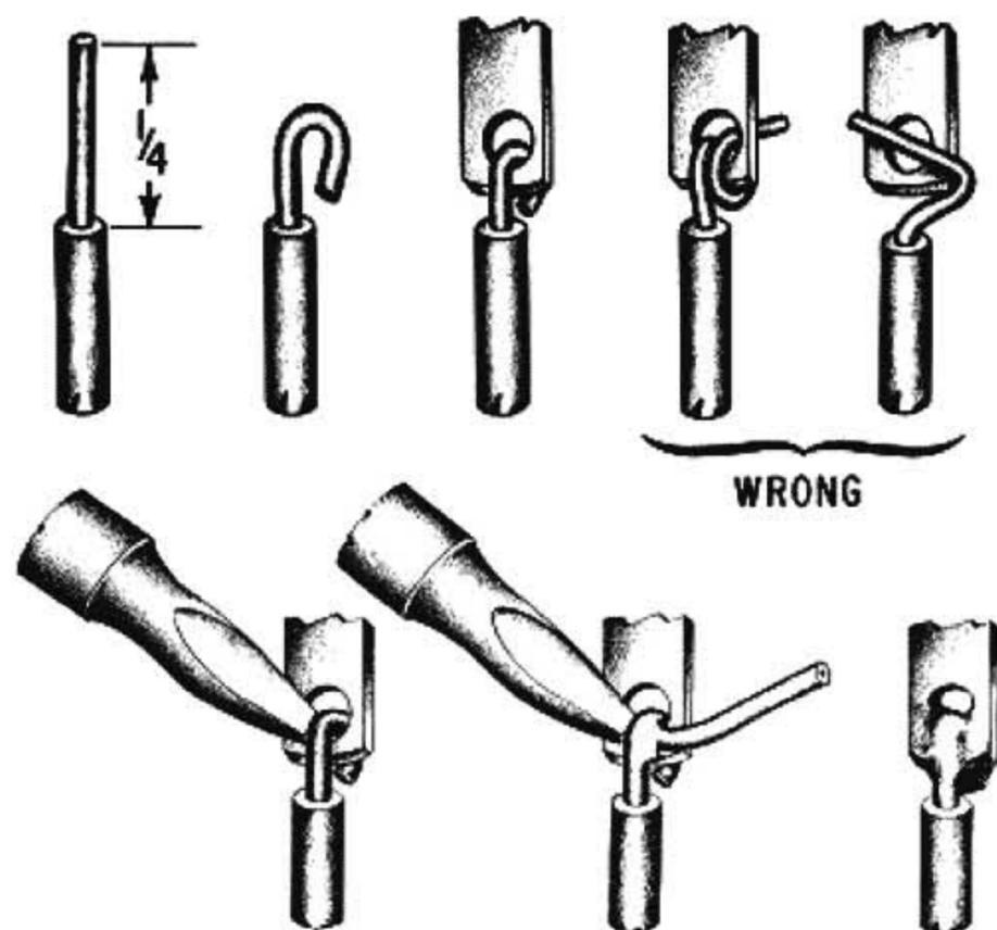
One of the best ways to make a good mechanical connection is to bend a small hook in the end of the wire, and then to crimp the hook onto the terminal lug. The amount of bare wire exposed need not be exactly  $\frac{1}{4}$ -inch, but if it is too long, the excess might touch another terminal lug or the chassis. Do not wrap the wire around the lug more than one time, as this makes the connection difficult to remove if an error is made.
