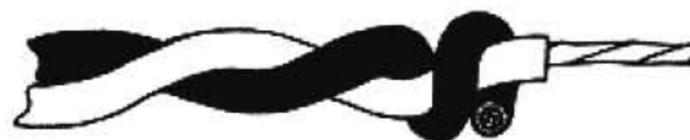
The lugs on switch CS are more fragile than the other lugs in this kit. Do not attempt to bend a hook in the end of the wire before inserting. Simply push the straight wire end in the lug hole, solder, and then cut off excess wire.
