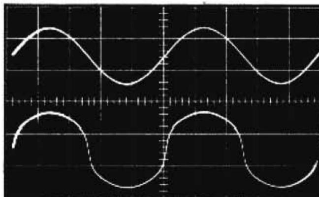
The rounded, rather than a squared or jagged, characteristic of this severely limited 200 watt signal in the Dynaguard-20 position maintains the best possible audio quality by minimizing extraneous harmonics. Input signal is upper trace.
