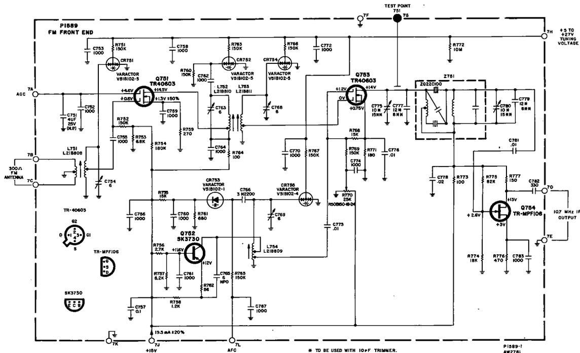
VOLTAGE & CURRENT MEASURED WITH ANTENNA TERMINAL SHORTED. ALL VOLTAGE  $\pm 10\%$  EXCEPT WHERE OTHERWISE NOTED.
