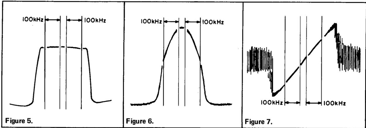
symmetry. Carefully adjust top and bottom core of Z304 for maximum gain and symmetry (see Figure 6). DO NOT READJUST Z302.
