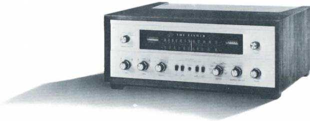
This superb receiver is identical to the 500-C described above, except that it also includes a high-performance AM tuner section. The AM circuitry features a high-gain pentode RF amplifier, a pentagrid converter, and an IF amplifier with switchable bandwidth. A front-panel switch selects either BROAD, for widest frequency response, or SHARP, for max-
