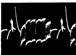
Q230 Emitter REC mode 50mV/10μsec. div.
