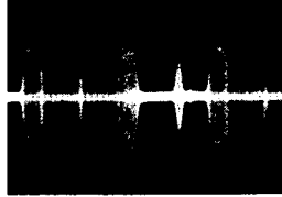
Q217 Emitter PLAYBACK mode 200mV/10μsec. div.
