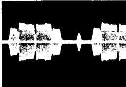
Q212 Base PLAYBACK mode 100mV/10μsec. div.
