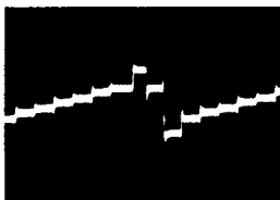
TP201 PLAYBACK mode 100mV/5msec. div.
