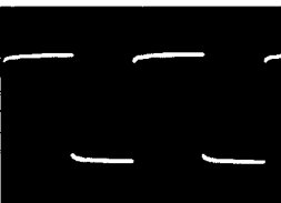
IC703 Pin (19) PLAYBACK mode 2V/10msec. div.
