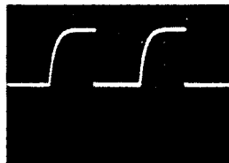
IC703 Pin (22) PLAYBACK/STILL mode 2V/5msec. div.
