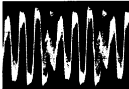
TP211 REC mode 200mV/0.2μsec. div.
