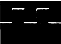
IC703 Pin (25) PLAYBACK/SLOW mode 2V/10msec. div.
