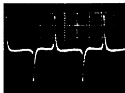
IC703 Pin (6) PLAYBACK mode 0.5V/0.5msec. div.
