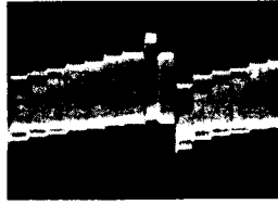
IC203 Pin (27) PLAYBACK mode 200mV/10μsec. div.
